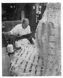
IN PARACHUTE LAB, Hal Widdows operates a heavy commercial-type sewing machine to alter a research chute. Nylon shroud lines are so firmly-woven the sewing machine needle must be air cooled.
